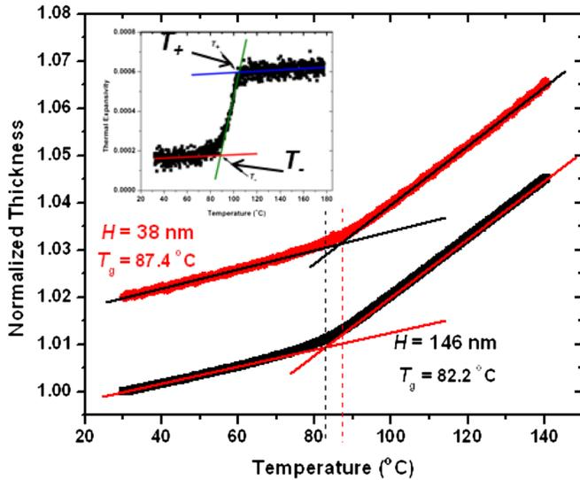
FIG. 1 (color online). Film thickness dependence on temperature, normalized by the thickness of the film at 30 °C, of star PS, 8 arms,  $M_w^{\text{arm}} = 10$  kg/mol films with  $H = 146$  nm and  $H = 38$  nm. The inset is the temperature dependence of the thermal expansion of the  $H = 146$  nm thick film.
