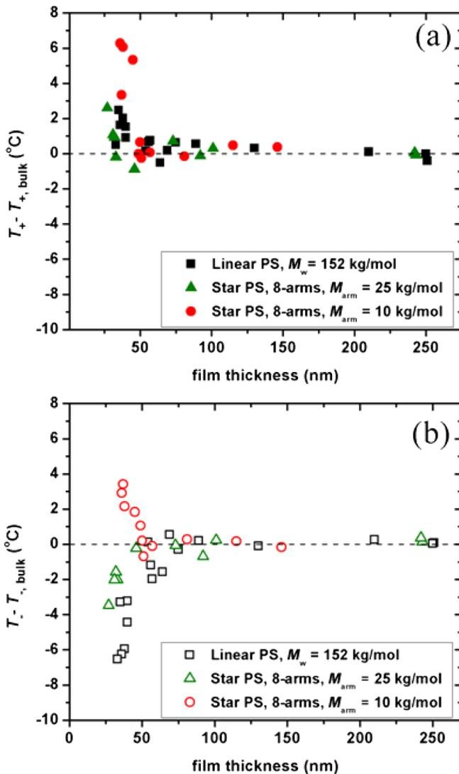
FIG. 3 (color online). Thickness dependence of (a)  $T_+$  and (b)  $T_-$  for linear PS, 8-arm star PS with  $M_w^{\text{arm}} = 25$  kg/mol, and  $M_w^{\text{arm}} = 10$  kg/mol.
