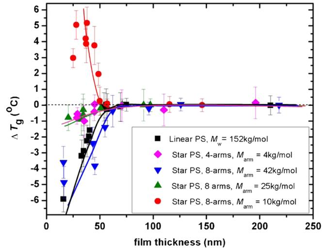
FIG. 2 (color online).  $T_g$ 's as a function of film thickness for linear PS (black squares), 8-arm star PS with  $M_w^{\text{arm}} = 42$  kg/mol,  $M_w^{\text{arm}} = 25$  kg/mol,  $M_w^{\text{arm}} = 10$  kg/mol, and 4-arm with  $M_w^{\text{arm}} = 4$  kg/mol. The lines are guides to the eyes.
