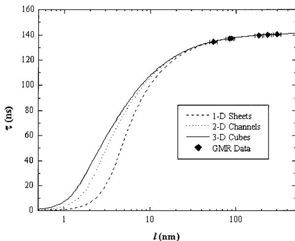
**Figure 2.** RTE model Ps lifetime vs mean free path,  $l$ , for three pore dimensionalities. Note that  $l$  is nominally a geometry independent measure of pore size, particularly for large pores.
