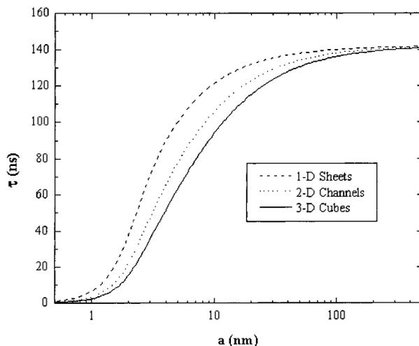
Figure 1. Ps lifetimes calculated with the RTE model vs pore size for three pore dimensionalities.
