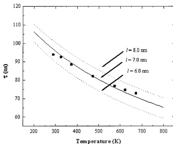
**Figure 5.** Ps lifetimes measured in a low-K porous silica film (Nanoglass A10B) as a function of film temperature and RTE curves (from ref 5).
