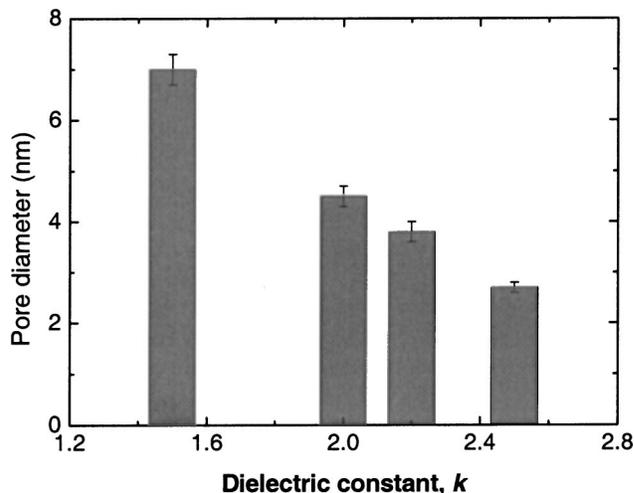
**Figure 7.** A trend between pore size and dielectric constant is observed in XLK films. Note the dielectric constant values were determined in the uncapped samples.
