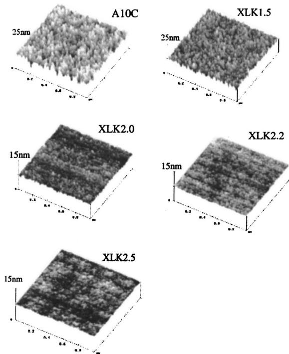
Figure 8. AFM images of the A10C film and the XLK series of films. Notice the difference in the scales. The depth scale of A10C and XLK1.5 is 25 nm whereas it is 15 nm for the other three films.
