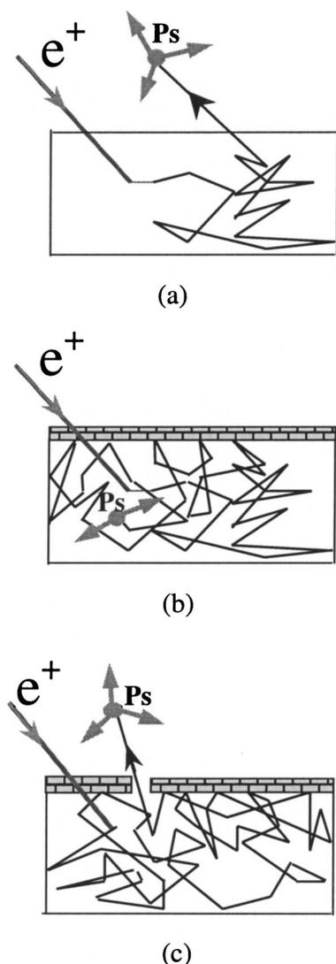
**Figure 1.** Ps behavior in barriered porous low- $k$  films with interconnected porosity: (a) no barrier, (b) an effective barrier, (c) a barrier with pinholes or discontinuities.
