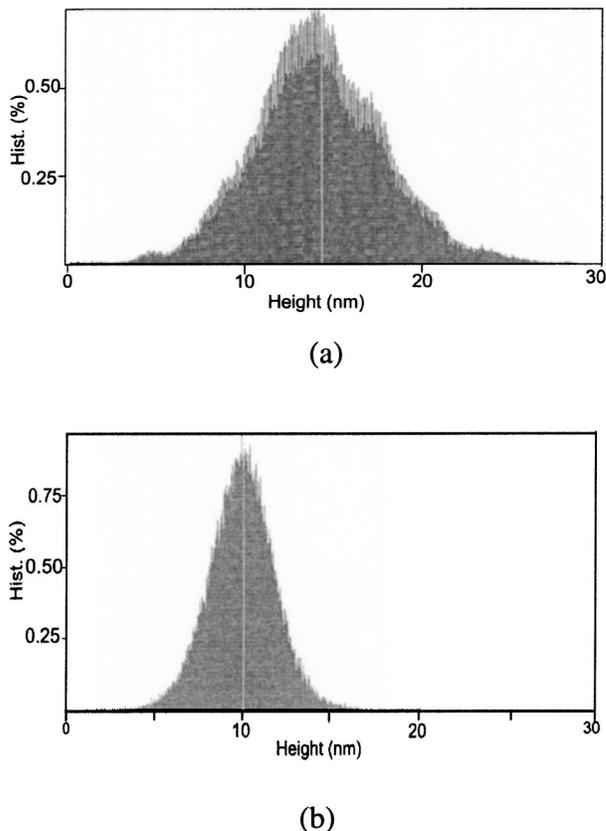
Figure 9. Histograms of peak height profile of (a) A10C and (b) XLK1.5 films based on their AFM images shown in Fig. 8.
