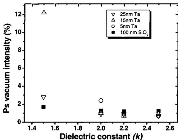
**Figure 4.** Ps vacuum intensity in the capped (100 nm SiO<sub>2</sub>) and Ta-barriered XLK blanket films at 5.0 keV beam energy.
