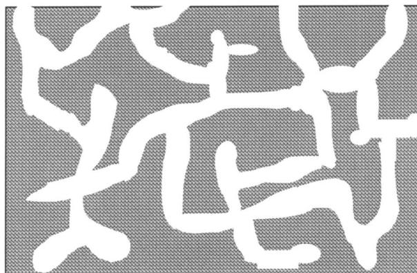
**Figure 6.** One possible example of a highly interconnected porous network which can be reasonably well characterized by an average tubular pore diameter.
