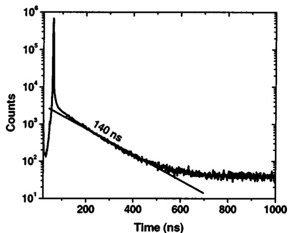
**Figure 2.** A typical PALS spectrum of the uncapped XLK films where virtually all the Ps decays with a single lifetime close to the vacuum value of 140 ns.
