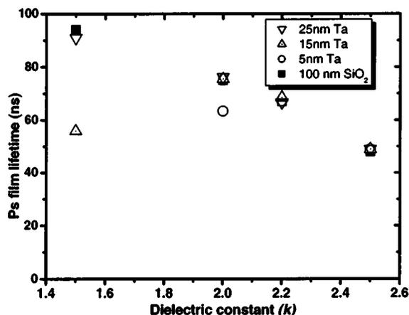
**Figure 5.** Fitted Ps film lifetime in the capped and Ta-barriered XLK films at 5.0 keV beam energy.
