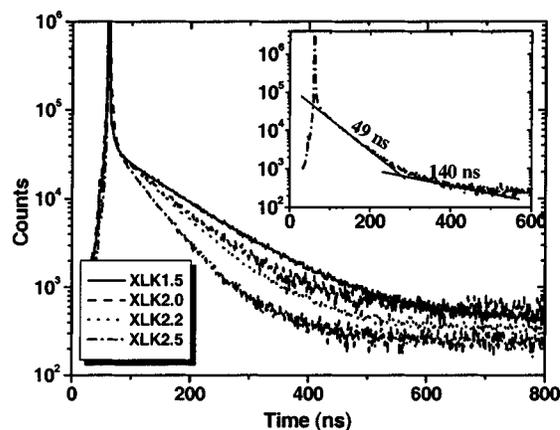
**Figure 3.** PALS spectra of capped XLK films. The inset spectrum of XLK2.5 is presented as an example to show that an intermediate lifetime component is required for acceptable fitting in the spectra of the capped films.
