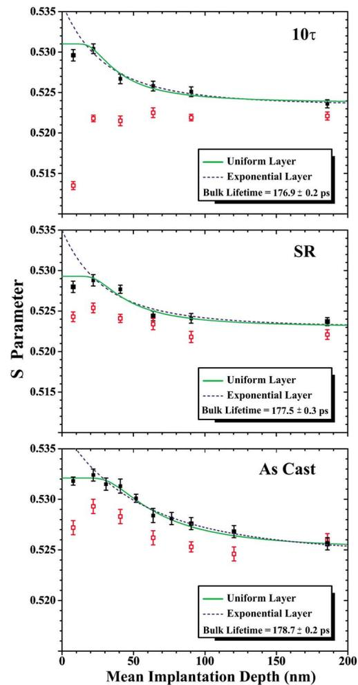
FIG. 1. (Color online) Depth-profiled Doppler broadening spectroscopy  $S$  parameter results for the  $10\tau$ , stress relieved (SR), and as cast samples. The  $S$ -parameter near the fatigue-fractured surface (solid symbols) is significantly larger than  $S$  for the undeformed face (open symbols) at equivalent depth. Fits of the depth profiles to simple models of  $S$  parameter depth dependence (uniform  $S$  layer—solid line and exponentially decreasing  $S$ —dashed line) are shown.
